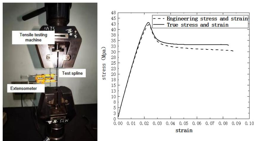
Figure 3. The CMT5105 universal electronic testing machine (*left*) and ABS material stress-strain curve. (*right*).
