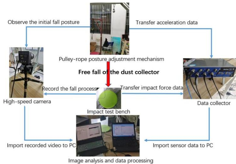
a) Drop/impact test process
