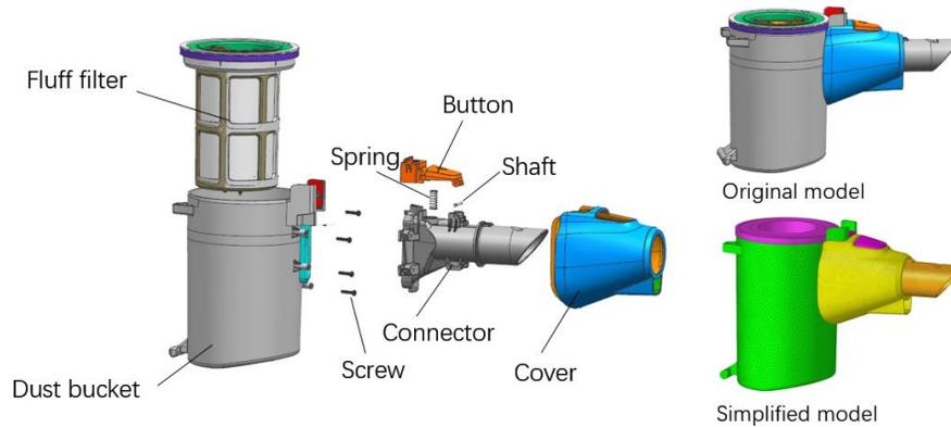
Figure 1. The structure of the dust collector (*left*) and the comparison between the original model and the simplified model (*right*).
