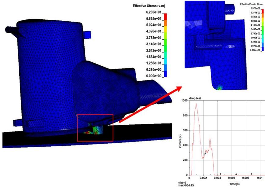
Figure 5. Stress and strain distribution and time history curve of impact force on the dust bucket in drop posture Q.
