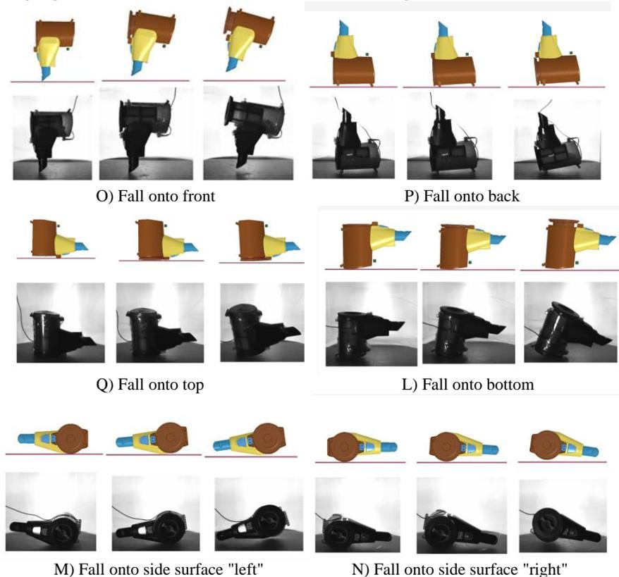
Figure 4. Comparison of impact process between numerical simulation and high-speed camera shooting.
