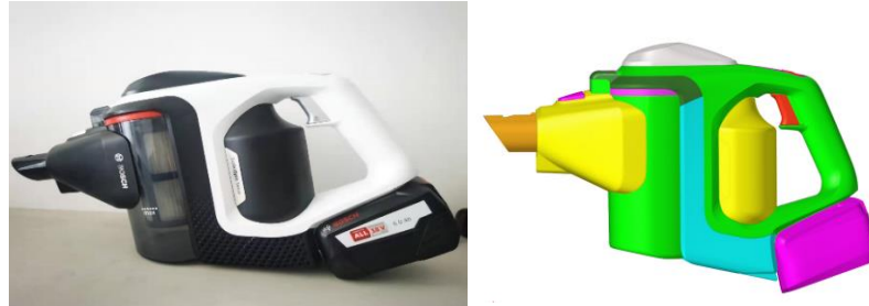
Figure 1. Host prototype ( left ) and finite element model ( right ).
