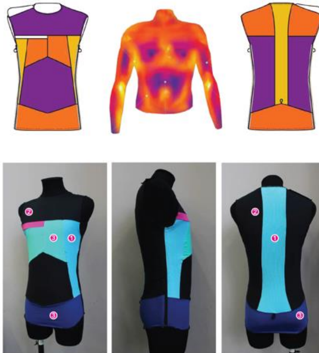
Figure 2. The inner layer (1- Maximum breathability and anti-odour effect with Dyamond X-Statics by Borgini Jersey; 2 - Warmth protected with Nilit Heat technology; 3- Maglificio Ripa's nanofiber, in two weight variants, guarantees thermoregulation).
