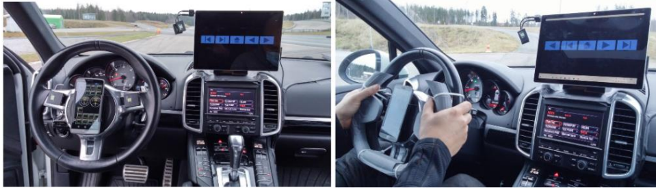
Figure 3. Placement of actuators, sensors, MS tablet and Origo wheel.
