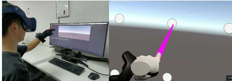
Figure 2. The pointing task based on HTC-Vive VR headset and Noitom HI5 gloves.
