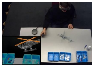
Figure 1. Illustration of the assembly workstation. A participant is performing the helicopter assembly task with the Magic Leap One. The participant's field of view is shown in the lower left corner. The next new component to be added is displayed in orange.
