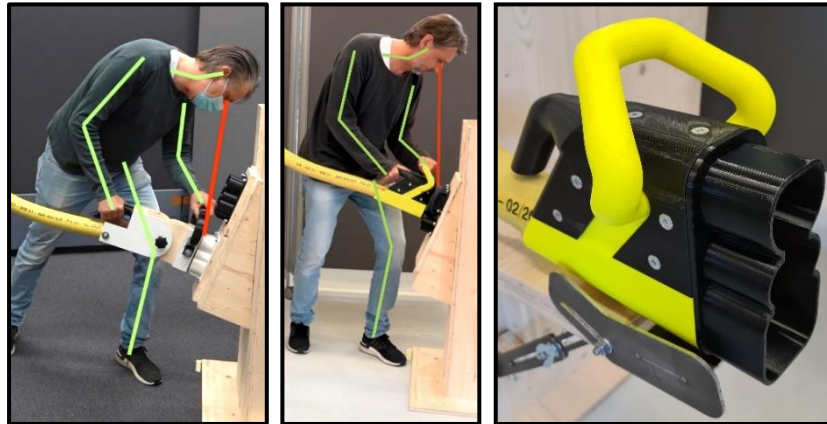
Figure 3. 98% man; left: using the first ergonomics model; center: using the improved model. Both sockets are within the identified comfort zone; right: improved connector design
