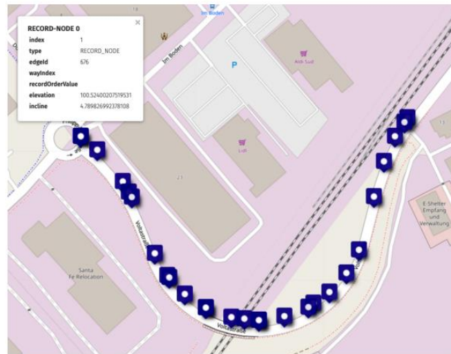
Figure 4. Visualization of the final computation and storage of altitude and incline data
