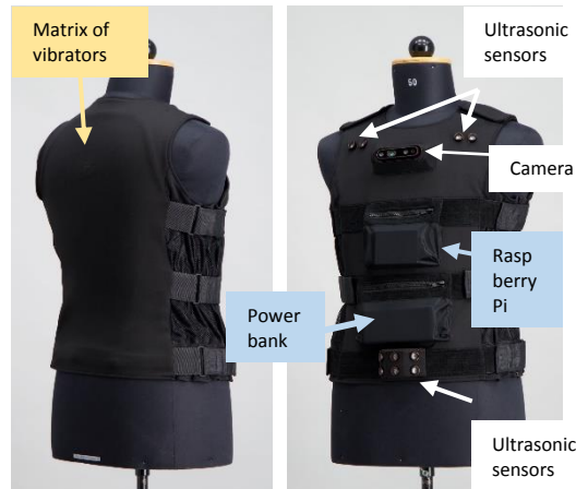
Figure 2. A developed AP systems fulfilling both a) for capturing environmental cues by sensors and b) having tactile interfaces toward the human receiver as well as powering and control.
