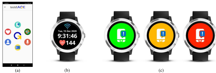
Figure 2: User interfaces of the sustAGE solution: (a) home screen of the smartphone app, (b) home screen of the smartwatch app, (c) display of the smartwatch app when receiving notifications (green), recommendations (yellow), and alerts (red).
