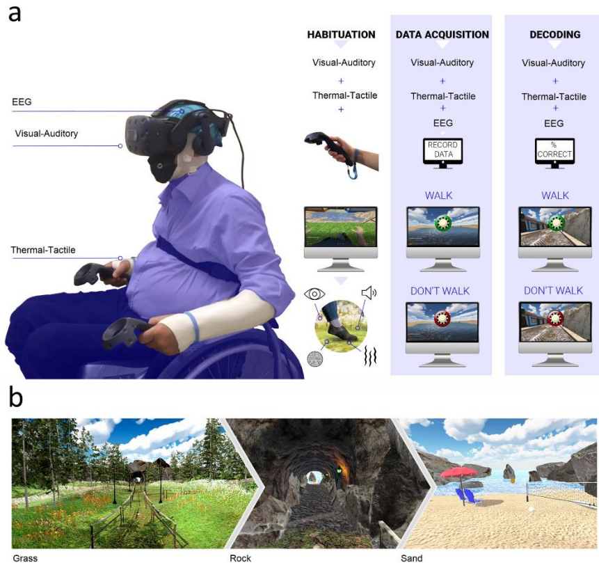
Figure 1. Experimental design and setup. a) During (Habituation) the subject controlled the avatar with the hand commands. In the second phase (Data Acquisition) EEG data was recorded while the subject was instructed to think about “Walk” (green cue) or “Don’t walk” (red cue). In the last phase (Decoding) neural activity was recorded and decoded in real-time. trials. b) Example of a complex scenario with multiple types of feedback. Visual, auditory, tactile, and thermal feedback were coherent throughout different modalities and scenarios.
