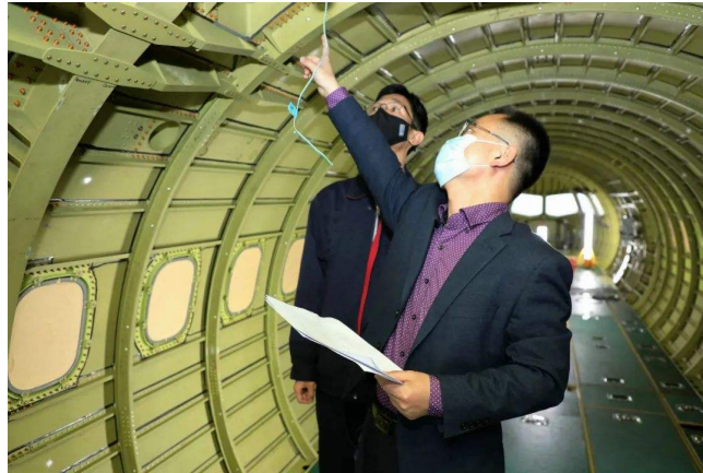
Figure 1: Zonal safety analysis on the real airplane.
