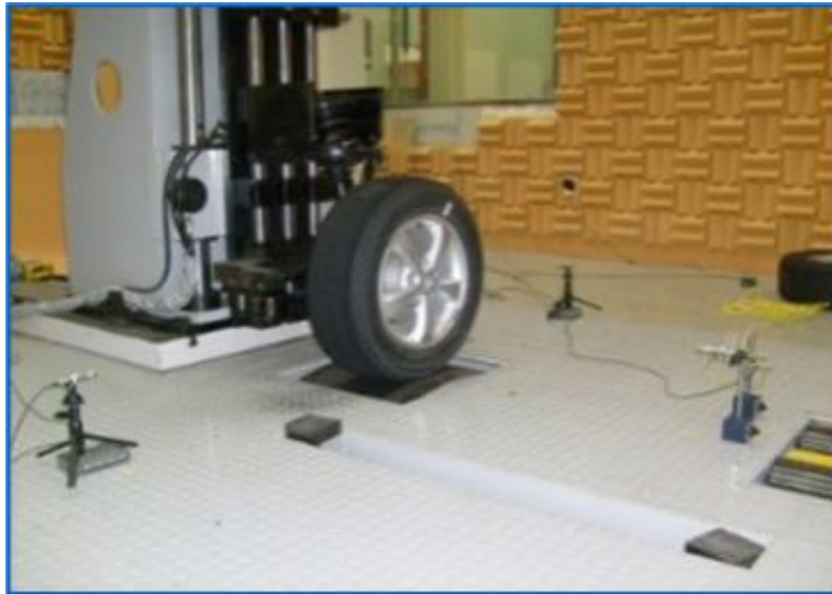
Figure 3: Microphone set up for measurement of tire noise
