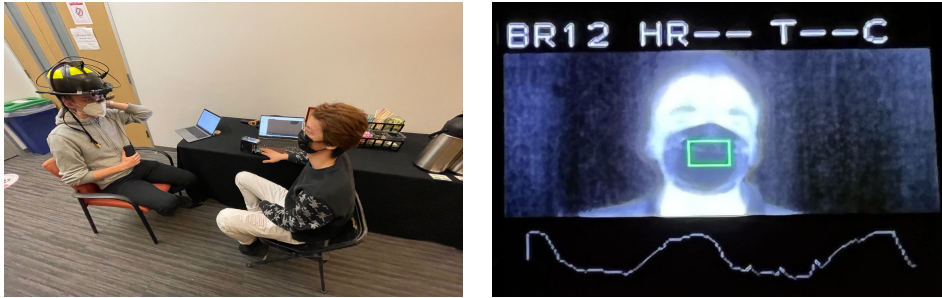
Figure 5: The lab test environment (left) and the thermographic display on HUD (right).
