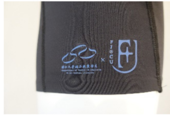
Figure 22: This photo shows a heat transfer label layout in the front flank of the left leg using high elastic adhesive film in the trousers' hem to improve wearer comfort.
