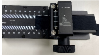
Figure 6: Bending test device to collect textile bending data.
