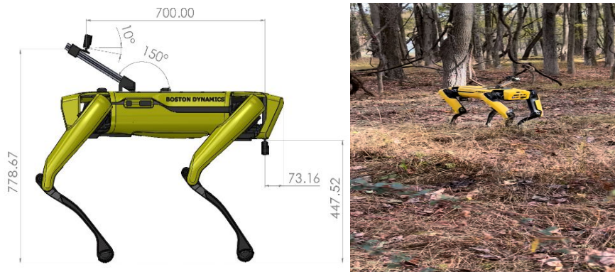
Figure 1: Spot Dynamic Robot System (Boston Dynamics Support Center, 2021), left image is CAD drawing of Spot, right image is Spot shown in wooded environment.
