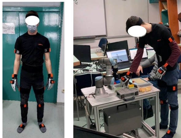
Figure 1: Xsens suit with sensors and human-robot collaborative workplace.
