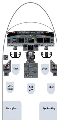
**Figure 5:** Internal layout of Cockpit Simulator.
