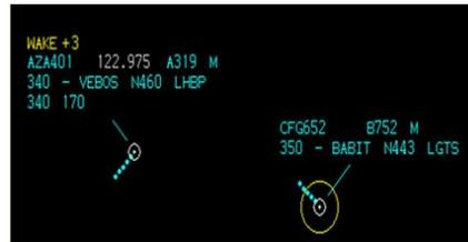
**Figure 1:** Wake alert displayed to controller.
