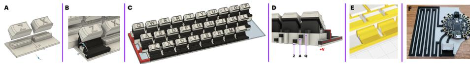
**Figure 2:** A) Constraining two non-conductive key parts next to one another B) Constraining the complementary conductive part C) Full keyboard layout D) Return electrode routing to the rear of the input device E) Separate .STL files in slicing software F) 3D printed pull down resistor and socket for direct microcontroller integration.
