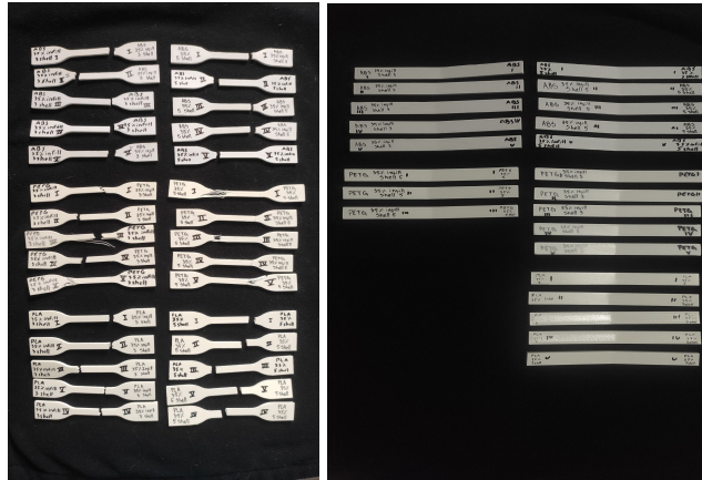
Figure 6: Tensile and flexural specimens after rupture respectively. (Authors, 2022).
