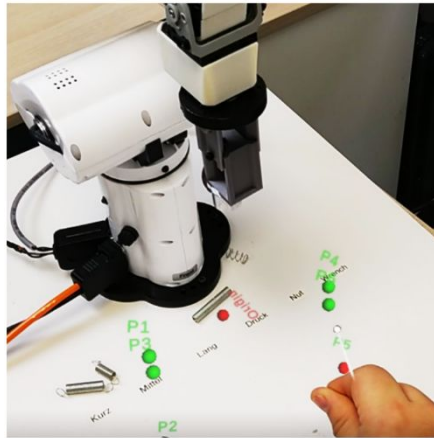
Figure 6: Robot operator is placing working points in the AR environment.
