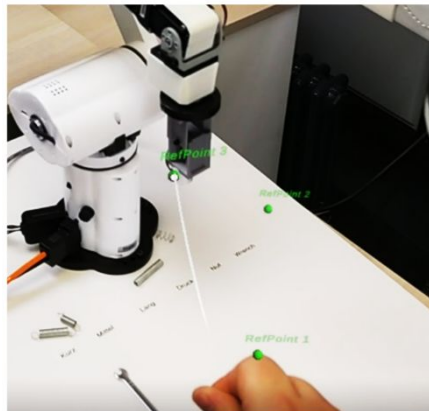
Figure 4: Robot operator is placing working points in the augmented reality environment.
