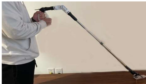
Figure 5a: Student demonstrating telescoping electromechanical reacher to grab object with joint at handle.
