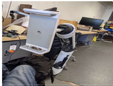
Figure 6a: Arm mounted on wheelchair with electronics holder attachment.
