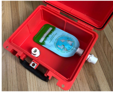
Figure 4a: Pressurized storage case holding liquid-food pouch and space for electronic controls and motor.
