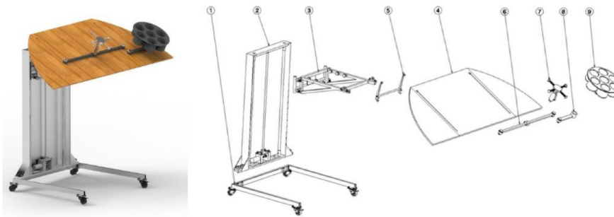
Figure 4: Overview of the painting table with its components (canvas and color cans supports).
