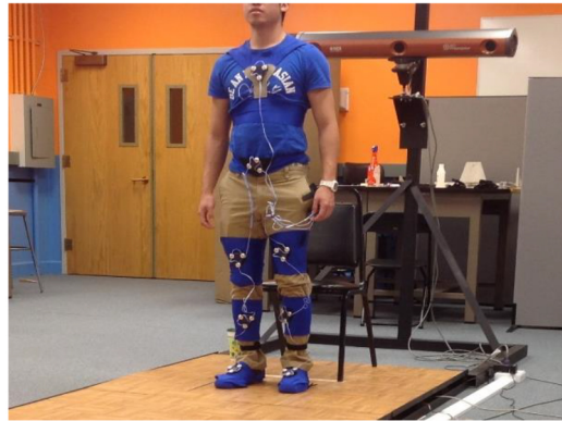
Figure 1: Showing a student subject instrumented with 8 rigid bodies, each having 3 markers attached.
