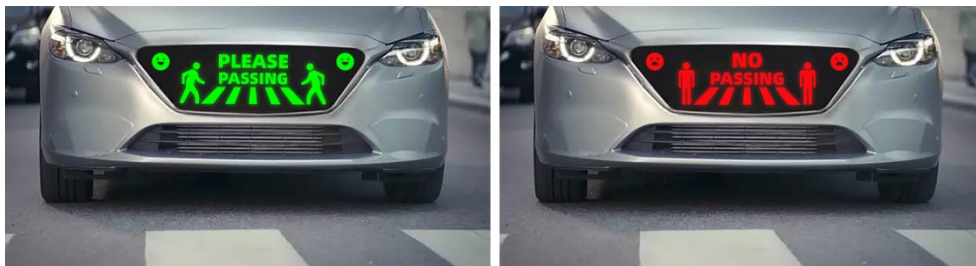
Figure 2: Design of external human-machine interface for automated vehicles.
