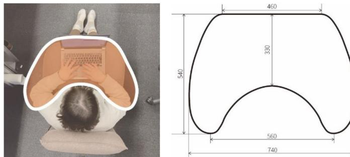
**Figure 2:** Size of the cushion model produced.
