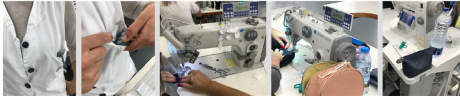
Figure 3: Operator using the device inside the pocket (two pictures to the left) and devices glued to sewing machines.
