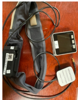
Figure 4: bandanas with simple electroencephalography and GPS device.
