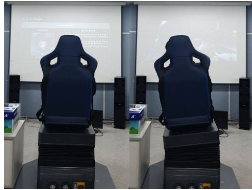
Figure 1: (Left) Neutral state of the motion simulator (0°) (Right) The state rotated 10° to the left of the roll axis.
