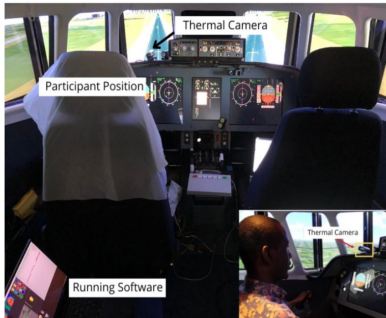
Figure 2: Illustration of the experimental setup. A participant sitting in front of the thermal camera mounted on the flight simulator cockpit. Thanks to the used algorithms, no chin-rest was used during the whole experiment, thus participants could move their heads freely.
