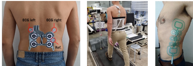
Figure 1: Left: recording multi-electrode array with approximate placement on the subject. Middle: A subject during the test with the multi-electrode array secured by an elastic girdle. Right: The ETA electrode.
