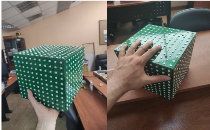
Figure 2: Proposed interactive die prototype.
