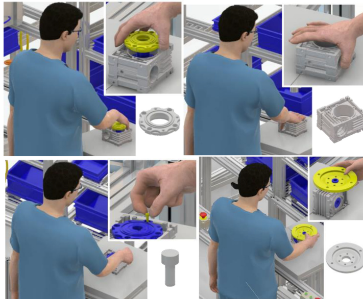
Figure 9: Examples of grasp results for different parts: a. Bearing cover. b. Housing. c. Screw. d. Flange.
