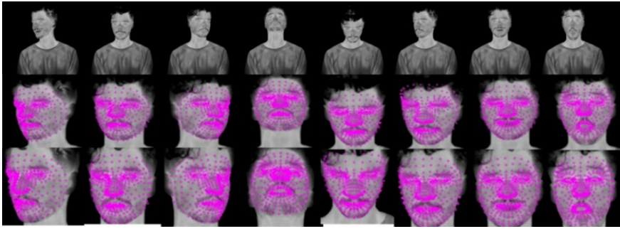
Figure 3: YOLO and Viola&Jones crops and mediapipe 468 landmarks on IR images with rotations and facial expressions. FLIR A35.
