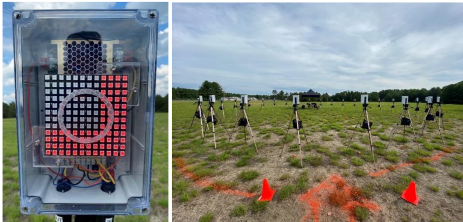
Figure 2: Example light box target with LED screen displaying a shape that represents an enemy threat (left), placed on stands in a 360-degree circle (right).
