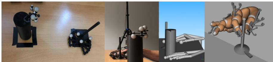
Figure 4: From left to right: cylinder ( d = 50 mm and d = 10 mm), starting position, visualization of the ART-FTM, visualization of our 6DOF target finger tracking.
