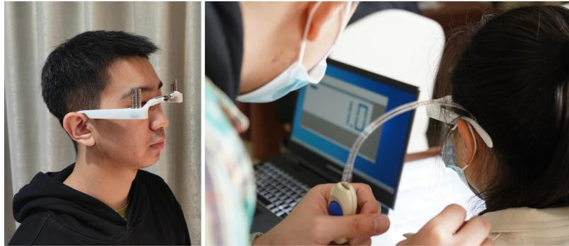
**Figure 2:** The process of experiment. (Left: The participant was wearing weighted prototype. Right: The clamping force was being measured).
