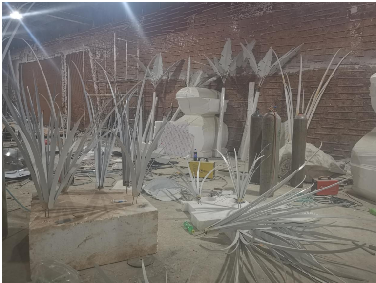
(Cutting shapes, assembly welding, polishing, painting of stainless steel materials).
