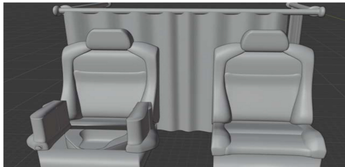
Figure 5: Car seat emergency toilet design from the front.
