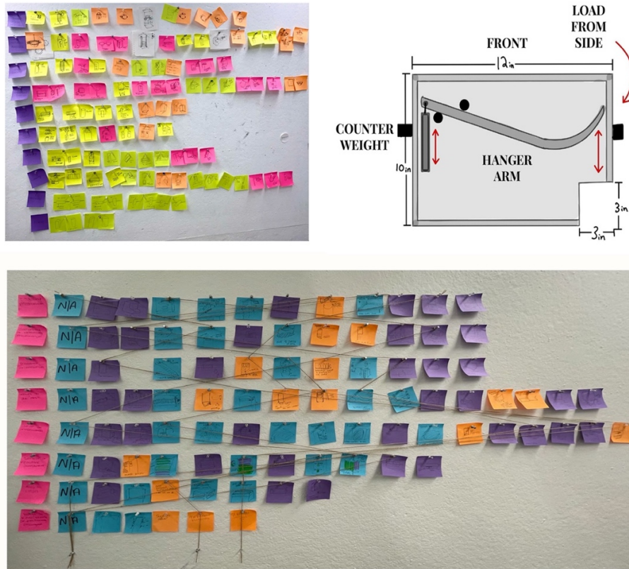
Figure 3: Examples of Thumbnail Concepts, Morphological Matrix Used to Map Concepts, and Example of Initial 2D Design Concept.
