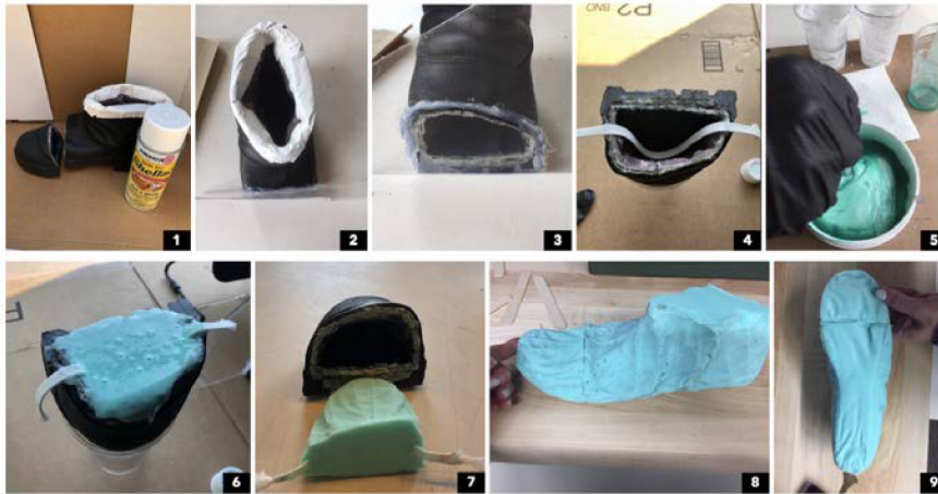
Figure 2: Process for capturing the fire boot interior.
