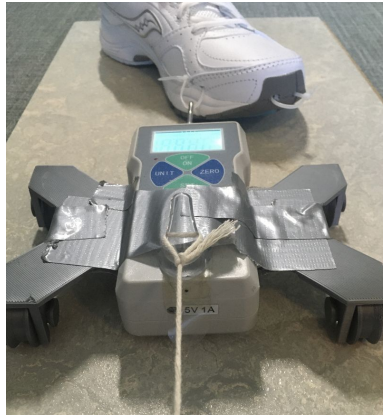
Figure 4: Data collection set-up for dry, normal foot strike, linoleum conditions.
