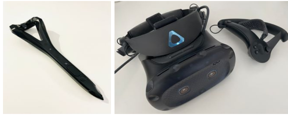
Figure 2: The VR apparatus: Logitech VR ink pen, HTC cosmos, and valve index Pro.
