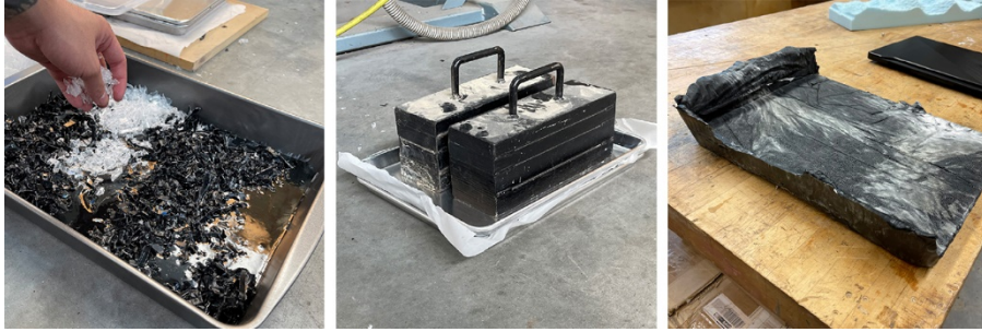
Figure 6: Layering plastic to form thick blocks for CNC milling. (Cong Khanh Vu, 2021).
