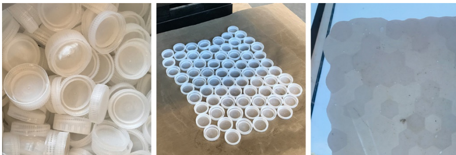
Figure 2: Melting water bottle caps into thin translucent honeycomb patterned sheets. (Taghreed Ayman Shalaby, 2021).
