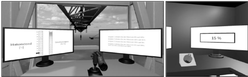
Figure 1: Experimental setups in the VR. Left: VR environment crane cabin, joystick, visualization of hand, visual feedback. Right: VR environment table, rotary control with knob, inclination 45°.
