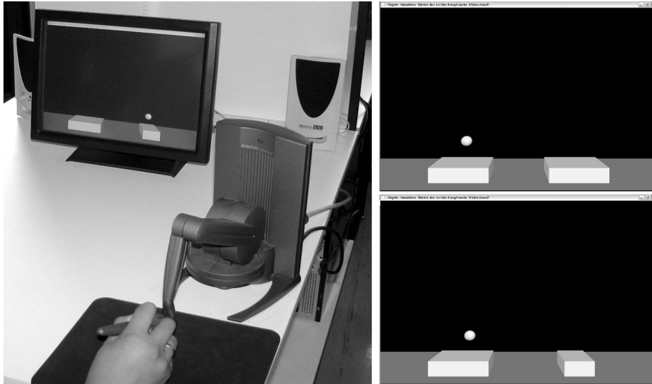
Figure 1: Experimental setup with screen and haptic display (left panel) for the size manipulation of the test key, as well as the two variants of the test key (large vs. small) and the virtual cursor (right panels).
