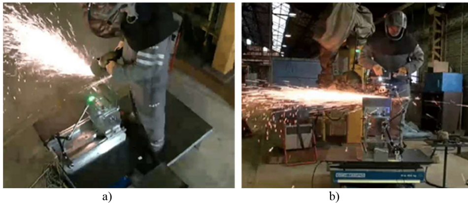
Figure 1: Experimental setup using different types of tool: a) traditional grinding tool and b) cobot.
