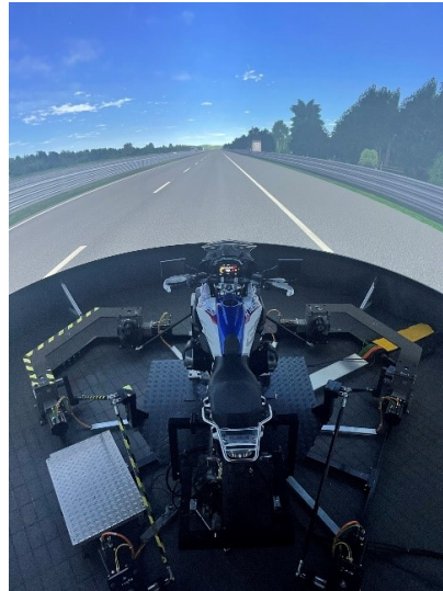
Figure 1: Motorcycle riding simulator mounted on a dynamic platform.
