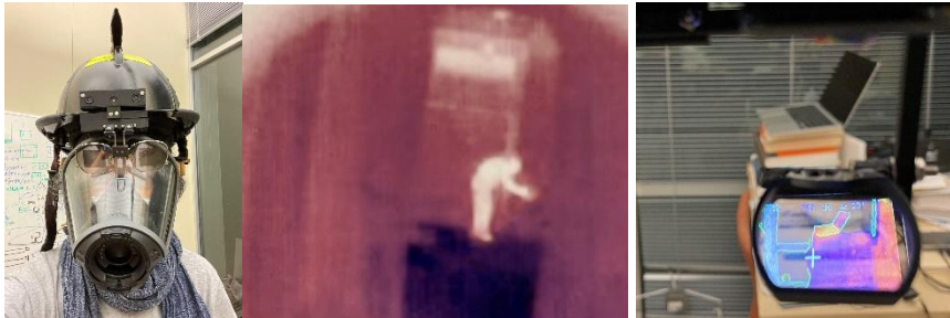
Figure 2: The EXR helmet (left), streamed thermal video (middle), and edge overlay (right).
