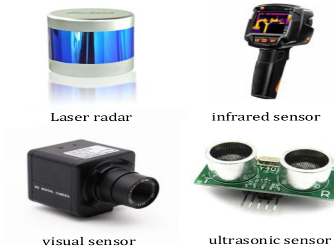
Figure 3: Surrounding environment sensing system.
